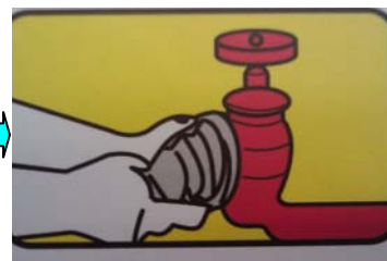
連接水帶 Connect the fire hoses
